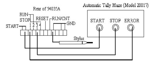
Figure 4: 54035A/20017 Connection diagram
