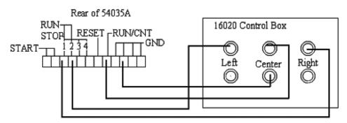
Figure 2: 54035A/16124 connection diagram
