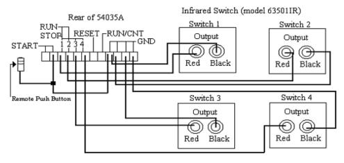
Figure 5: 63501IR/54035A Connection Diagram
