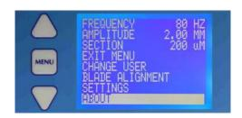
Use the  $\triangle$  or  $\nabla$  keys to scroll to the line 'ABOUT' and press the MENU key.
