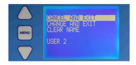
Use the  $\triangle$  or  $\nabla$  keys to scroll to the line (in the example shown) 'USER 2'. Pressing 'MENU' again will cause the 1<sup>st</sup> letter of the name to be highlighted. The rotary knob can now be used to scroll through the alphabet to select a new letter or symbol. Press the  $\triangle$  to confirm and move to the next letter position; use the rotary knob to select a new letter. ( $\nabla$  selects the previous position). Continue until the new user name is acceptable.
