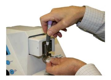
The blade should be fitted by loosening the two screws on the arms of the holder and sliding the blade under each washer and pushing it firmly back against the rear stops. The screws should not be over-tightened. See the illustration above.
