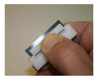
The blade is now safely gripped with its cutting edge protected from damage and can be safely handled during the fitting operation with minimal risk of personal injury.
