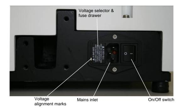
Voltage supply selector (example shown is set to 220-240V)
