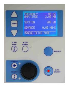
Press the 'SLICE ON/OFF' key to commence the cut. The 'SLICE ON/OFF' key will now change to a red illumination. Use the rotary knob to control the advance speed as the blade moves through the tissue. (Note that, if desired, the advance speed can be reduced past zero and
