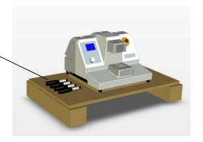
3. Screw four carrying handles into the instrument base. Ensure the handles are fully screwed in.
