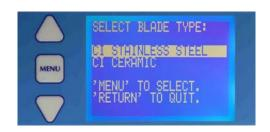
You must now choose which type of blade you want to calibrate. Scroll to the appropriate blade using the  $\triangle$  or  $\nabla$  keys and press 'MENU' to select.
