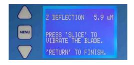
The display will now change to that shown on the left. Note that the uppermost line shows the current Z axis (vertical) deflection. At this point it indicates zero because the blade is not moving.
