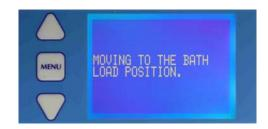
Press the 'LOAD BATH' key and the display will change to that shown. The bath table will be moved to its lowest position to allow a specimen bath to be loaded (or an existing one removed).
