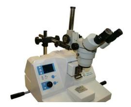
7000smz fitted with the stereoscopic microscope
