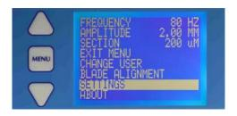
From the basic menu screen use the  $\triangle$  or  $\nabla$  keys to scroll to the line 'SETTINGS' and press the MENU key.
