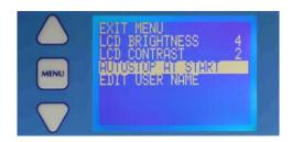
Use the  $\triangle$  or  $\nabla$  keys to scroll to the AUTOSTOP line. Press the MENU key to toggle between AUTOSTOP AT END or AUTOSTOP AT START. Use the  $\triangle$  or  $\nabla$  keys to scroll to line EXIT MENU and press the MENU key to get back to the basic menu display.
