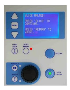
The automatic slicing process may be halted prematurely by pressing the 'SLICE ON/OFF' key in which case the display will change to that shown. Follow the instructions on screen to CONTINUE or ABORT the procedure. Pressing 'MENU' at this stage will allow access to menu functions permitting changes to frequency and amplitude etc.
