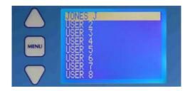
When the instrument is switched on the display will be as shown, showing any personalised user slots. This screen can also be accessed from the main menu.
