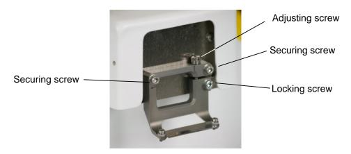
Fit the blade holder as shown and tighten the two upper securing screws. The lower locking screw should be tightened sufficiently to just grip the lower portion of the blade holder.
