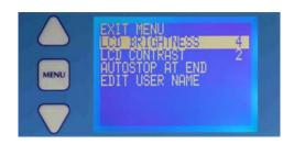
Use the  $\triangle$  or  $\nabla$  keys to scroll to line required and press the MENU key. The feature value will be highlighted and may be adjusted using the  $\triangle$  or  $\nabla$  keys. Press the MENU key to confirm the change.
