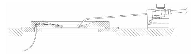
**Figure 10: Positioning the Suction Needle**
