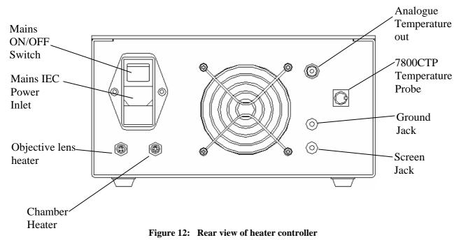
The green outlet is available to provide an electrical earthing point. It is connected internally to the earth
