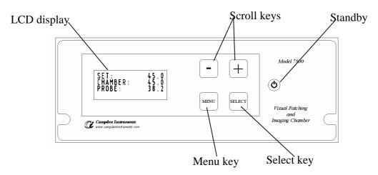
Figure 13: Controller front panel (as used with a slice chamber)
