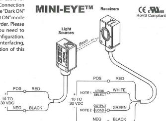
Note 1: Dark "ON" Operation: Terminate To Positive Light "ON" Operation: Terminate To Negative
