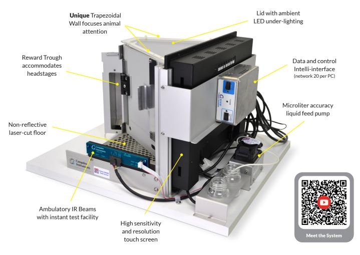
The Bussey-Saksida Chamber has always featured a **unique trapezoidal wall shape** in order to focus the animal's attention and facilitates the efficient and high-throughput cognitive evaluation of rodents. The chamber is **easily reconfigured** to a modular square arena with panels, levers, lights, and a range of other operators.
